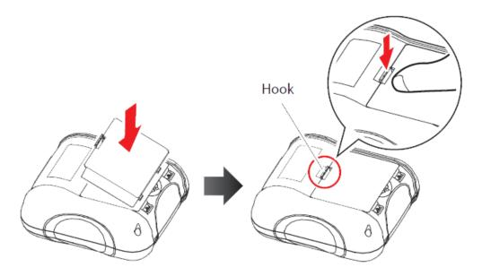
2. Insert the Printer roll in the correct orientation as indicated:
