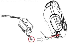
**4.** Ensure the power supply is switched on, then press and hold the power button for 5 seconds to switch on the printer:
